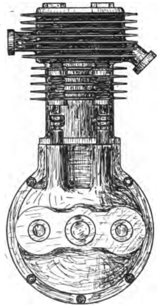
FIG. 13.—MOTOR-CYCLE ENGINE WITH AN L-HEADED AIR-COOLED CYLINDER. VALVES BOTH ON SAME SIDE OF CYLINDER.
